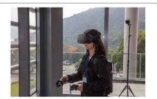
**Fig. 2** The learner with the VR gear. The learner worn the VR gear adopted in the ViSi—the computer backpack, headset and a pair of the trackers. The sensor is situated at a diagonal position to sense the motion
