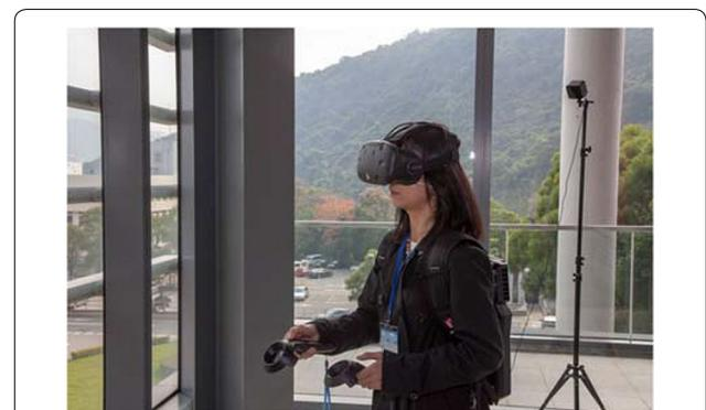
**Fig. 2** The learner with the VR gear. The learner worn the VR gear adopted in the ViSi—the computer backpack, headset and a pair of the trackers. The sensor is situated at a diagonal position to sense the motion
